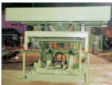
▲ INSTALLATION OF ATTACHED TYPE OF TURNTABLE AT HYUNDAI MOTOR
